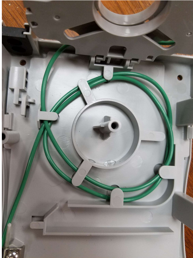
Slack of the loose tube unit in the slimbox base
